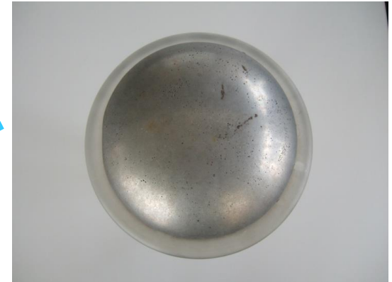
Top electrode: Few discharge craters
