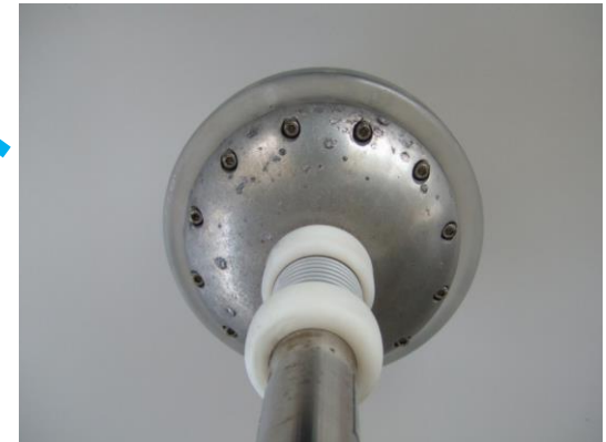
Bottom electrode: Many discharge craters
